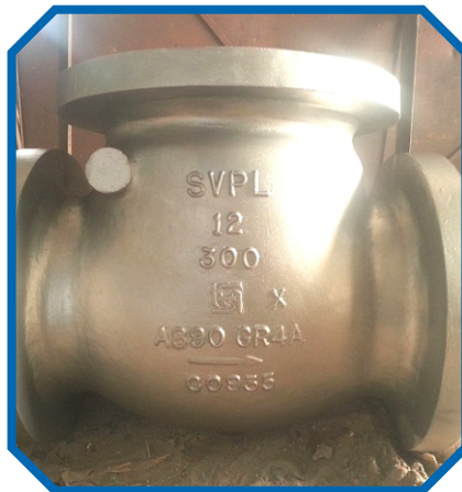
12" x 300 # SCV Body ASTM A 890 Gr. 4A
