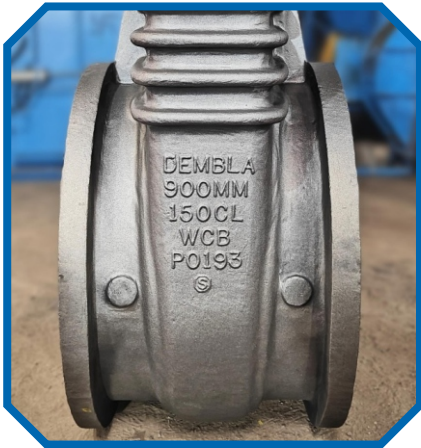
36" x 150 # GTV - WCB 100% Area RT at level 1
