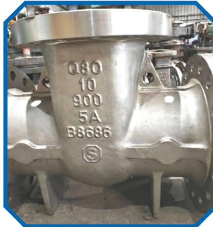
10" x 900 # GTV Body ASTM A 995 Gr. 5A
